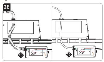
Connect flexible conduit or Romex to junction box with the proper fitting.
